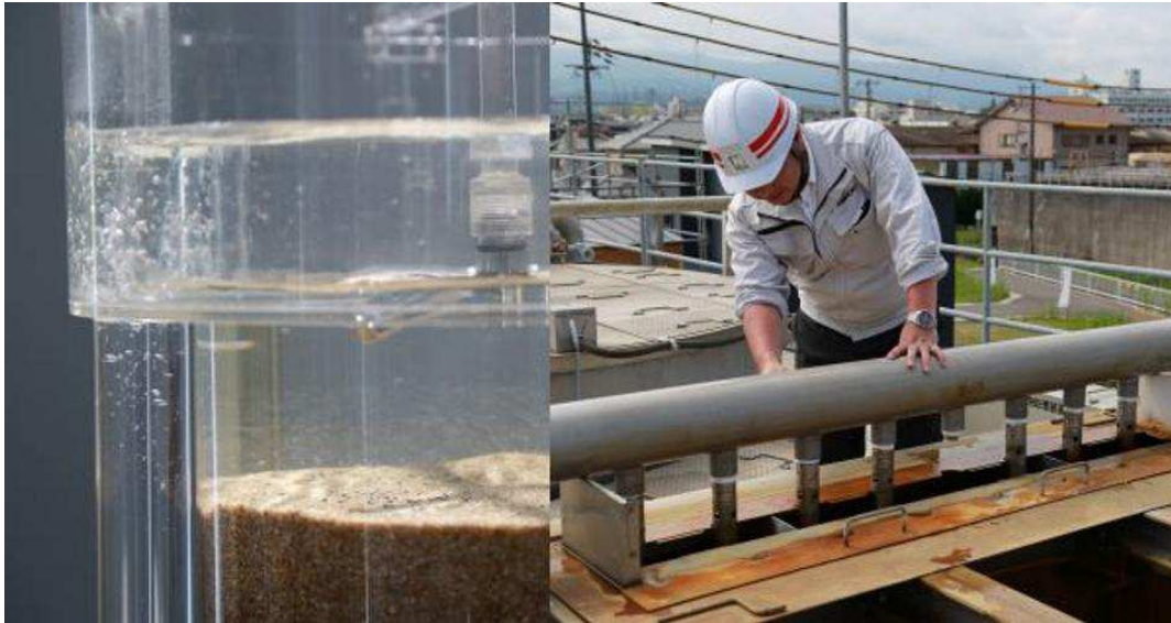
Chemiles relies on oxidation and contaminant-consuming bacteria to remove excess iron, magnesium, and ammonium nitrates. JAPAN BRANDVOICE
