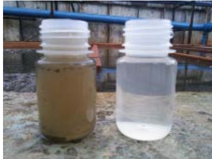
Grand Textile's raw water (left) and water purified by activated carbon (right)
