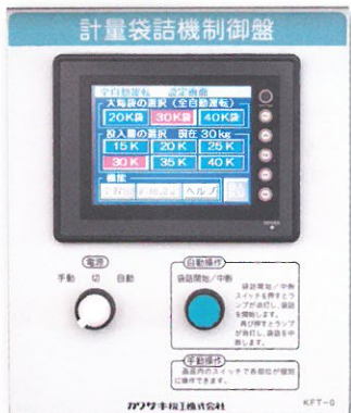
Packing machine control panel
