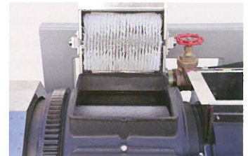
Rotating brush prevents clogging
