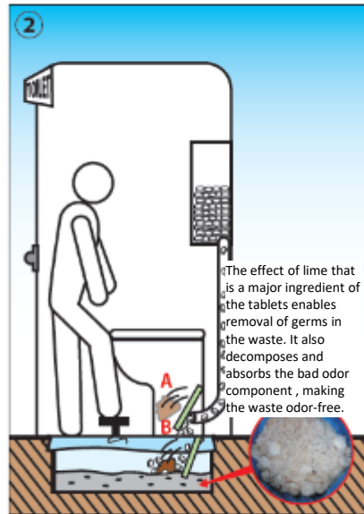
(2) Once you step on the pedal after defecation, valve A opens so that the waste falls onto valve B . At valve B , the waste is mixed with tablets of Mt. Fuji Toilet , then falls due to its own weight into the plastic container placed below. At the same time, new tablets are supplied onto valve B .
