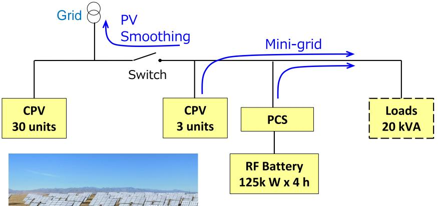
Switch ON: Grid connected model
