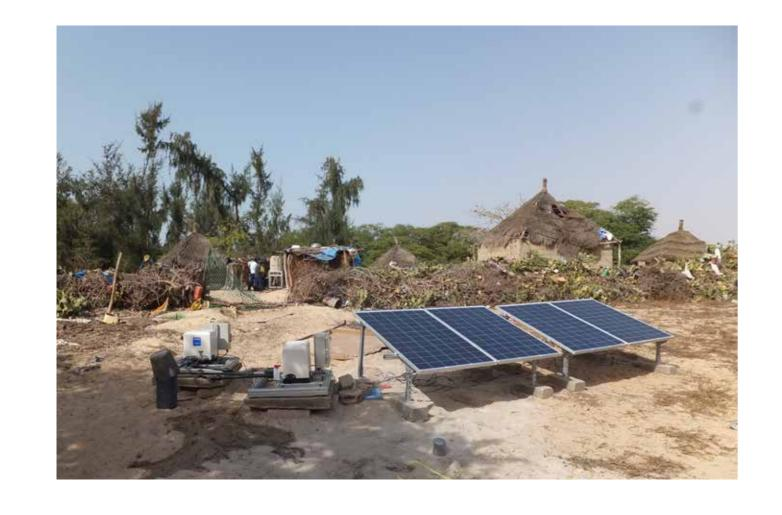
Teral's solar pumps directly utilize the DC power generated by solar panels without intermediate conversion to AC.
