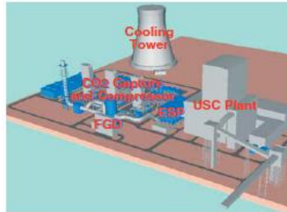
Result of FS on 500 MW USC + CCS
