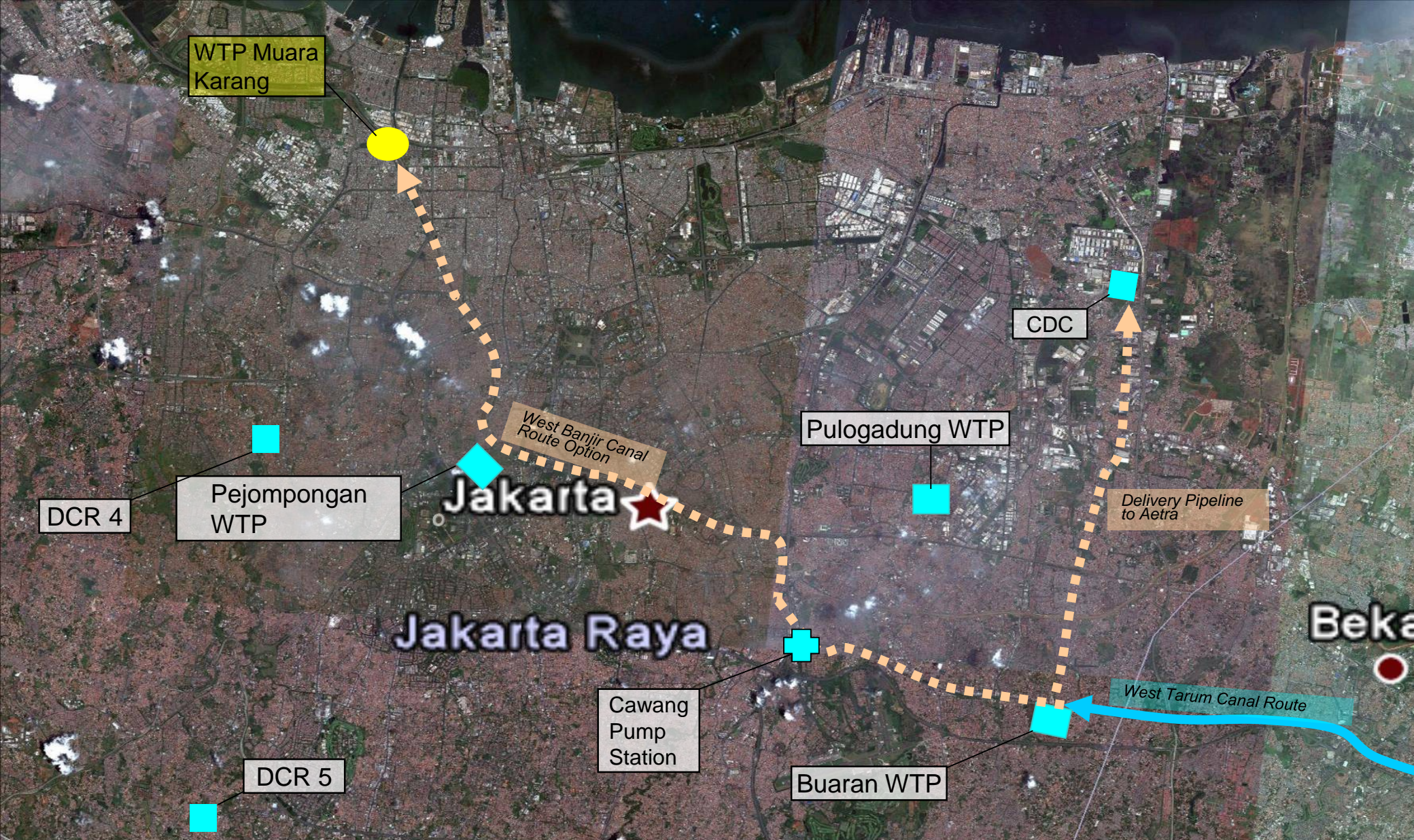
Jakarta existing water storage & required scheme delivery points
