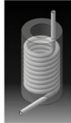
Cylindrical shape Cold Plate (For Motor and Tank cooling)
