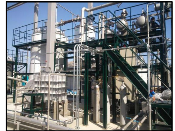
「The machine generates recycled oil from waste plastics.」
